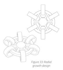
Each smaller ring connects two larger ones. The increased number of connection links causes the structure to somewhat resist folding, though it is still flexible and movable.
