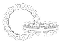
Figure 7: The disks "riveted" on these links add both acoustic and tactile properties.
