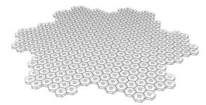
Figure 39: Hexagonal fabrics can be thought of as polar arrays instead of grids, leading to snowflake-like shapes.
