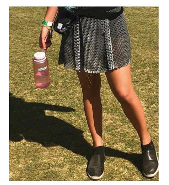
Given HP MJF's efficient XY speed, connecting flat panels is the most efficient approach to creating the skirt. The panels were tapered to create a basic, flattering, five-panel skirt. Each panel was then lined with a thicker, twisted chain to create smooth edges and easy attachment points for final assembly.
