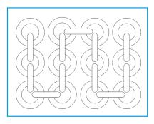
Figure 3: You can also design chains folded for compact packing and for printing parts that are longer than the print bed's dimensions.
