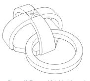
Figure 41: The quad fabric's tiling unit consists of a square with legs and a connector on the bottom right edge.
