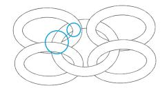
Figure 11: Ensure sufficient gaps to prevent accidental fusing
